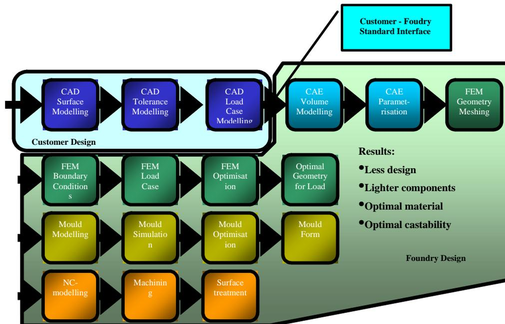
Figure 1. Design process of cast parts
