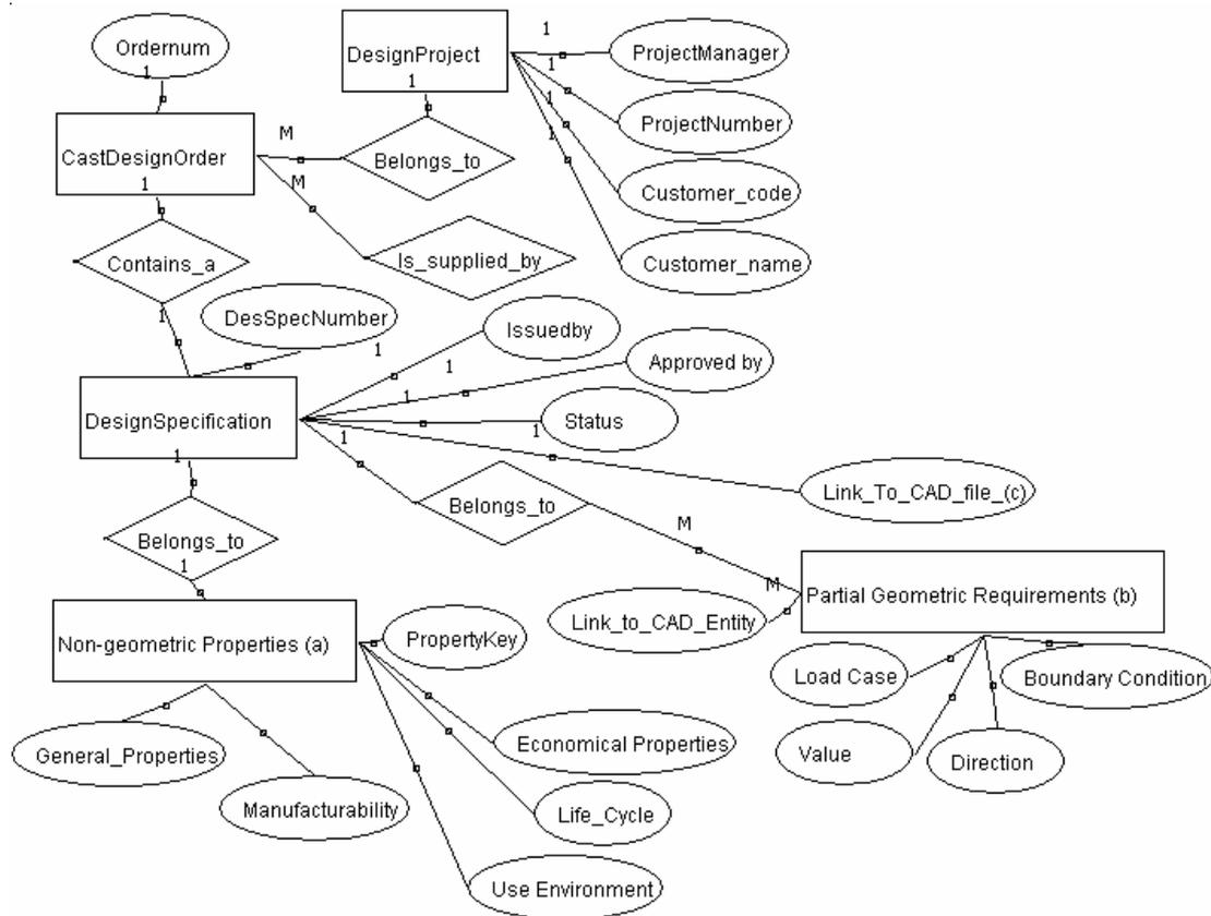
Figure 4. Customer cast design and manufacturing order main level ER-model.
