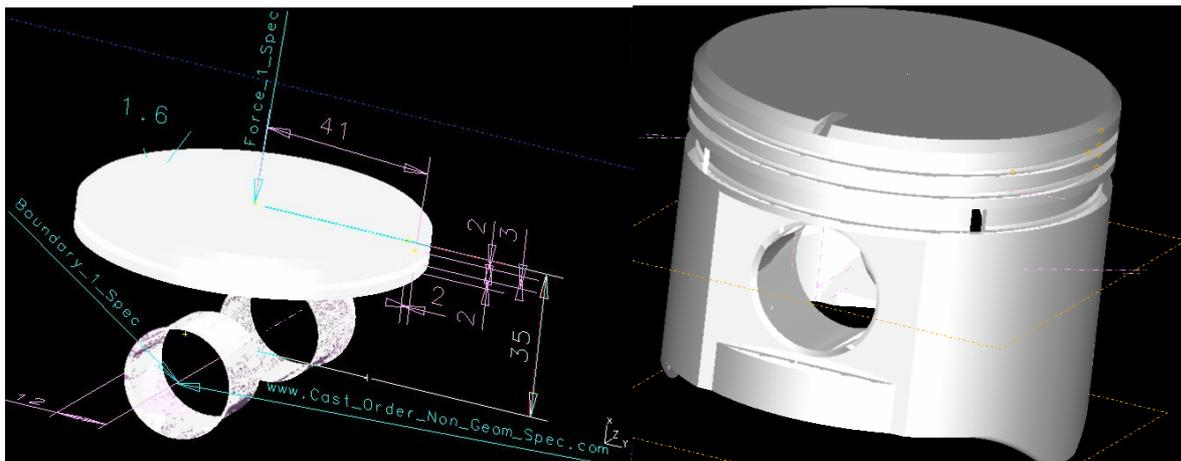
**Figure 9. a (left) Example of surface model based design specification model with URL-links to XML-database. b (right) Final product model after foundry related detail design.**
