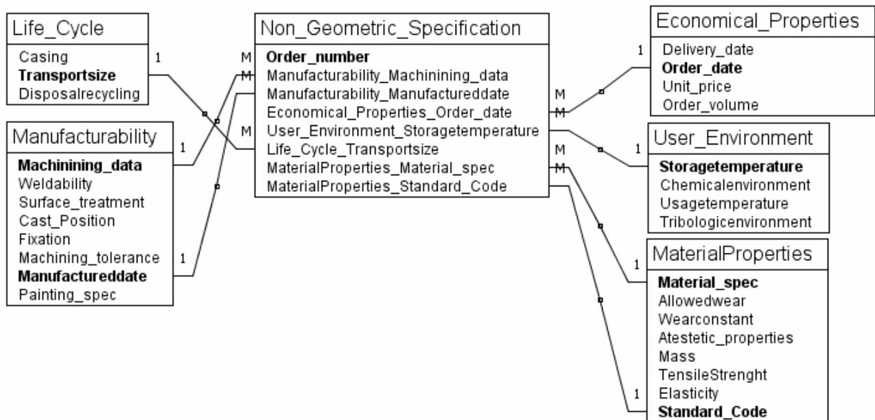
Figure 7. Non-geometric detail level data relation model, created from ER-model in fig. 5.
