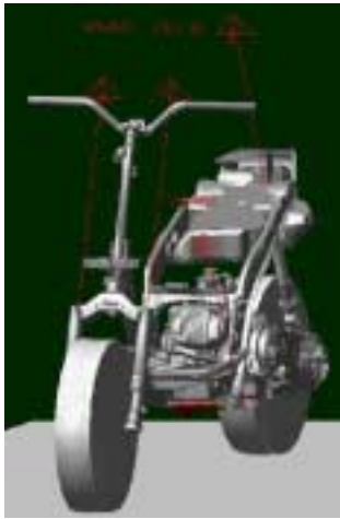
Figure 10. Forces acting on front (-) and rear (- -) wheel axes obtained by a drop-test simulation
