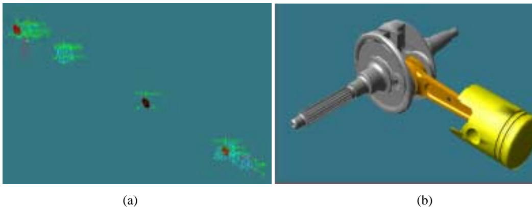
Figure 7. Multi-body representation of the engine crank mechanism of Figure 6: (a) functional scheme, (b) nominal geometry for visualization
