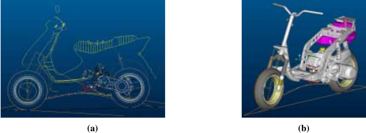
Figure 8. CAD model a two-wheeled vehicle: (a) skeleton model, (b) feature-based assembly
