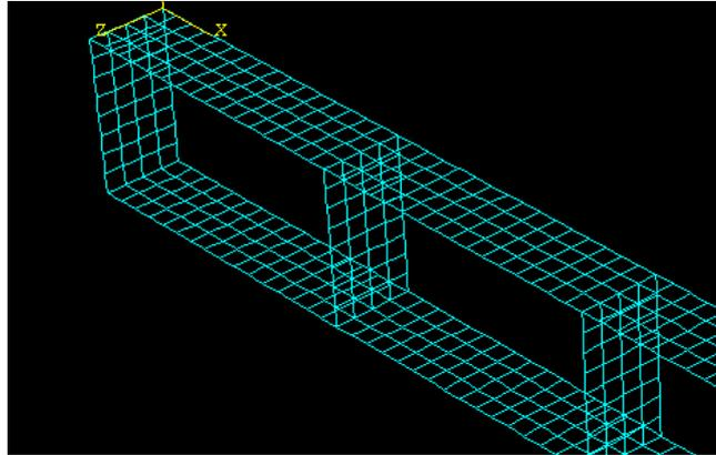
**Figure 7. Element meshing applied to describe the beam**
