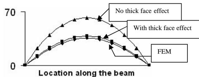
Figure 6. Beam displacement in mm
