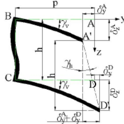
Figure 4. Deformed half segment
