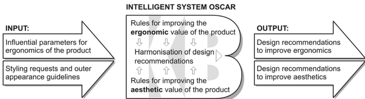
**Figure 4. Basic structure of the intelligent advisory system Oscar**
