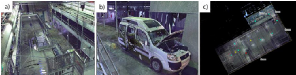
Figure 7. a) Rendered image of the point cloud. b) The high density of point cloud allows nearly photorealistic 3D visualization directly. c) A 2D layout of the measured space.
